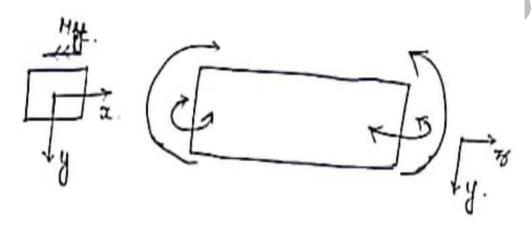
$$\frac{\partial q}{\partial s} = -t \frac{\left(I_{xx}V_x - I_{xy}V_y\right)}{\left(I_{xx}I_{yy} - I_{xy}^2\right)} x - t \frac{\left(I_{yy}V_y - I_{xy}V_x\right)}{\left(I_{xx}I_{yy} - I_{xy}^2\right)} y$$
